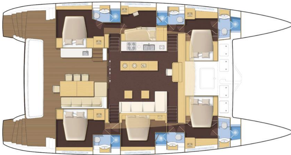
Cuisine centrale, 6 cabines / Central galley, 6 cabin version
